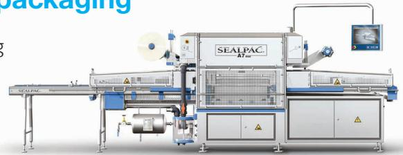
**Sealpac's traysealers are driven by high-quality servomotors that ensure a smooth packaging process.**
